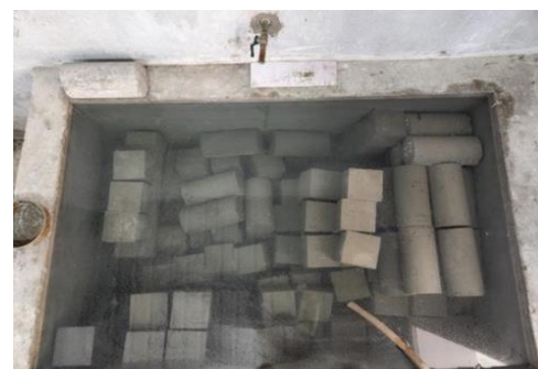
Fig 3: Concrete Cubes in the Curing tank
