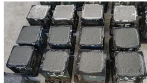
Fig 2: Concrete Cubes in the molds
