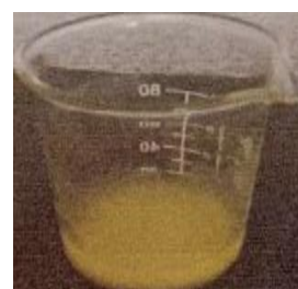
Fig-7: Nicotine dipicrate Precipitation
