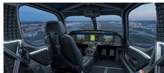
Fig. 4: Interior cockpit environment showing acoustic treatment panels, ergonomic seating, avionics displays, and simulation interface.
