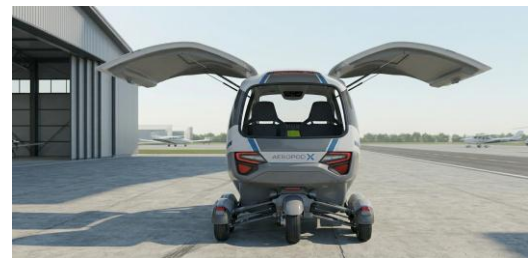
Fig. 3: Exterior operational visualization showing deployed roof panels and hydraulic stabilization system.
